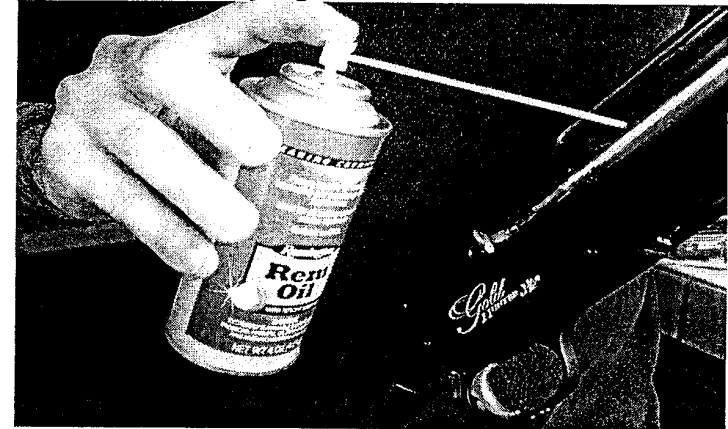
Figure 15: Spraying Rem Oil in chamber
